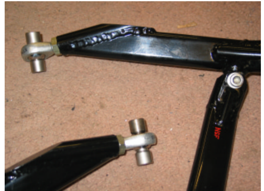
The improved track control arms, fitted with M14 rod ends.
